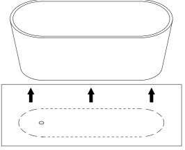
Fit plug waste into bath outlet, seal & tighten as required.
