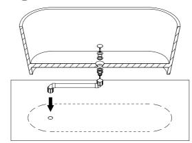
Fit out drainage connection to underside of bath. Position bath & connect drainage to floor waste.
