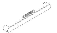
Place the fixing bracket on the circle that was marked in step 2. Use the pencil to draw a small circle as shown below. The power cord is to be fixed on the right side.
