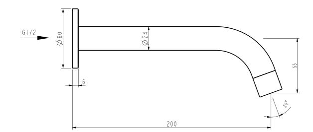
Slide the back plate onto the spout - make sure that the rubber is firmly in place to protect the spout and stop the back plate from moving around
