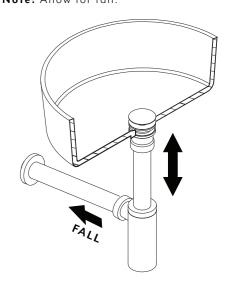
Engage kee seal into 40mm socket.
