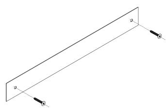
Fix magnetic strip to backing plate.
