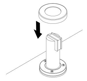
5 Fix catch to door using fixings provided.
