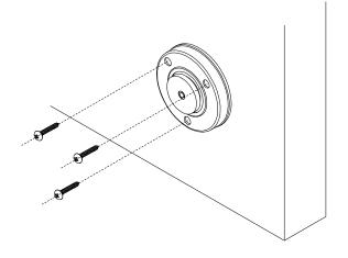
Fix stop to floor using fixings provided.
