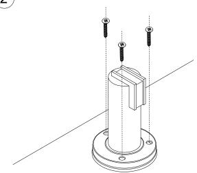
Mark out desired position for door catch in relation to door stop magnet on floor. Drill pilot holes into door.
