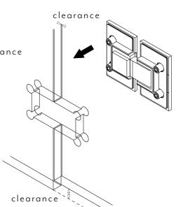
Fit hinge plate and packers with fixings provided.
