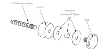
Use a temporary adhesive to stick one plastic washer to the barrel. Hold glass in place using special grips and screw the cap (with plastic washer and screw sleeve) through the glass and into the barrell. Tighten using standoff tool to clamp glass.
