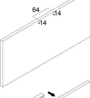
Drill holes into marked out positions. Check accuracy of distance of holes with hole positions in handle.
