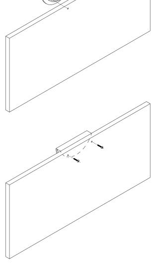
Fix handle to drawer/door using fixings provided.
