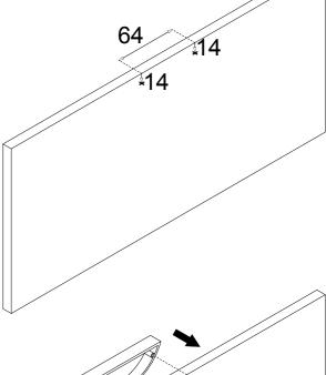
Drill holes into marked out positions. Check accuracy of distance of holes with hole positions in handle.
