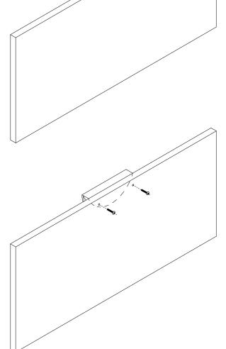
Fix handle to drawer/door using fixings provided.
