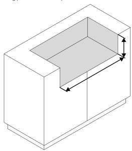
Cut the bench-top using the external measurements of the sink perimeter in conjunction with the desired sink overhang and cabinetry shelf.
