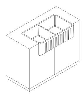
Install the benchtop & apply adhesive to sink perimeter.
