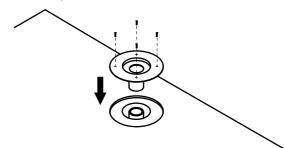
Adjust the top of the puddle flange to the finished height required for the shower grate installation.
