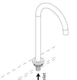
Connect pipework to inlet of spout.
