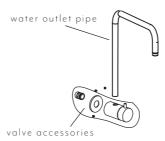
Put the straight arm into the holder, value accessories and wall seat, use M5 screws. Install the water outlet pipe into the top.
