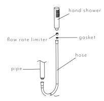
Make sure each screw connection is strong. Open the drainage system and water supply, check if theres any leakage in the connections.
