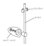
Before installing the hand shower, open and clean the pipe. Connect hand shower with the hose and the pipe
