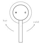
If the handle is still loose after tightening, remove the spindle and unwind in the bedded thread, retry again until firm grip is achieved.
