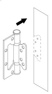
Pix hinge to door using fixings provided. Check door swing direction prior to fixing.
