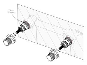
Slide the dress plate over the sleeve and press against wall.
