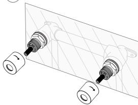
Install handle by using the allan key provided and tighten grub screw.
