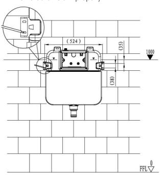
2 Drilling and installation of expansion screw
